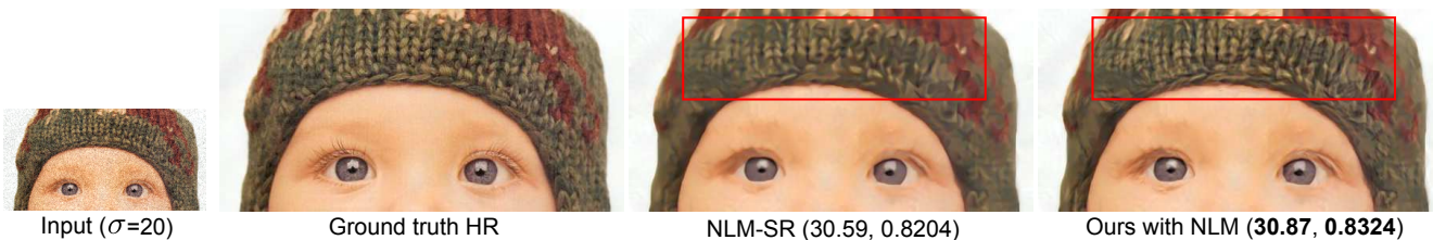
Figure 10. Baby . The woolen cap in our result is significantly richer in texture as compared to the conventional NLM-SR approach. The numbers in bracket denote (PSNR in dB, SSIM).
